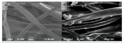
**Microencapsulation:** SEM images of (a) control cotton fiber; and (b) cotton fiber embedded with PentaHerbs microcapsules (1000×).
